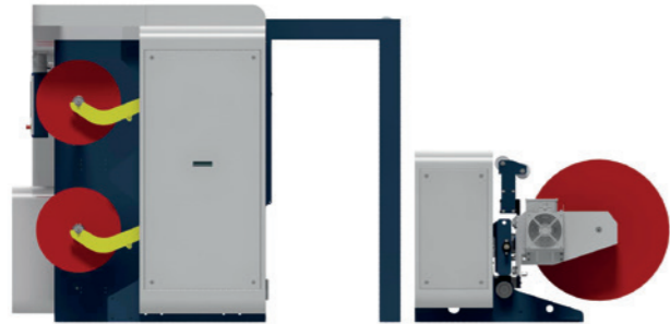
D Overhead web path: rewind on the opposite side of unwind
