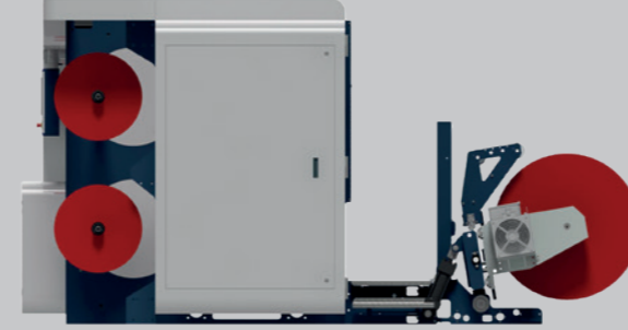
C+ Web passage under running board: semi-independent unwind stand
